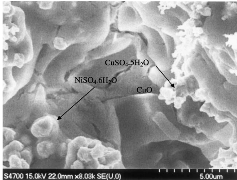
Fig. 9. SEM micrograph of the surface of a copper anode containing 2 w% Ni passivated in an electrolyte containing 160 \text{ g l}^{-1} \text{ H}_2\text{SO}_4 , 40 \text{ g l}^{-1} \text{ Cu}^{2+} and 40 \text{ g l}^{-1} \text{ Ni}^{2+} at a bath temperature of 60^\circ \text{C} . \text{CuO} , \text{CuSO}_4 \cdot 5\text{H}_2\text{O} and \text{NiSO}_4 \cdot 6\text{H}_2\text{O} are indicated by arrows.
